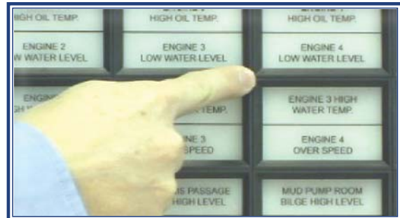
10- Push the corners of plastic bezel
